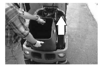
13.Clean the inside of the hopper compartment by scraping any compacted debris with a scraper. Use a stiff broom or brush to clean the vacuum screen.
