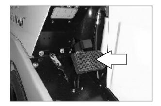
3. Move the throttle lever back into the Idle engine speed position.
