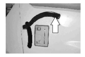
2. Press the water pump switch to the middle off position.
