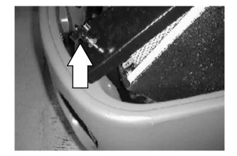
5. Remove the hopper dust filters from the machine.
