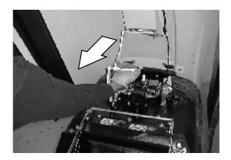
4. Unscrew the dust filter housing cover bolts, and open the dust filter housing covers.
