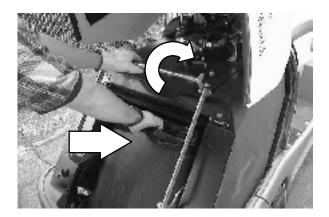
18. Hold up the hopper cover while pushing the prop rod in.
