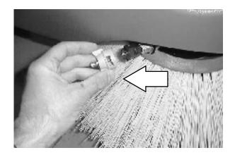
3. Remove and clean the spray nozzle filter screen.
