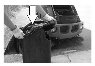
15. Insert new bag and liner, or debris hopper if not using bags, back in the machine.
