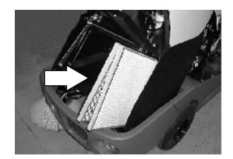
9. Close the dust filter housing covers and secure with the housing cover bolts.
