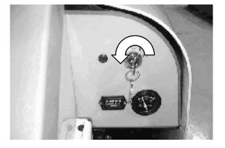
6. Turn the ignition key clockwise until the engine starts.
