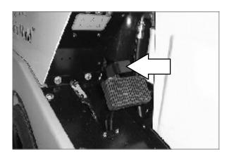
5. Turn the machine power off. Remove the switch key.
