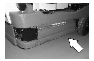
Check the engine air filter dust cap.
