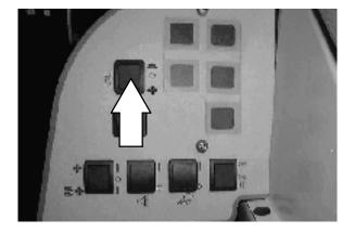
3. Press the vacuum fan/side brushes switch to the middle off position.
