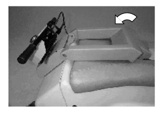
7. Turn the steering assembly knob clockwise until steering assembly is secure.
