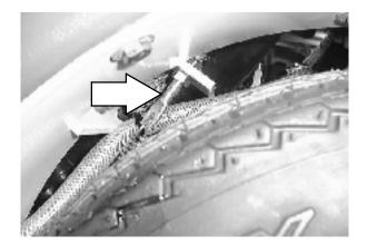
The side brush should be replaced when it no longer sweeps effectively for your application. A guideline length is when the remaining bristles measure 75 mm (3 in) in length. You may need to replace the side brush sooner if you are sweeping light litter or use a brush with shorter bristles if you are sweeping heavy debris.
