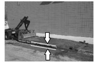
3. To winch the machine onto the truck or trailer, attach the winching chains to the rear tie down locations. The rear tie-down locations are located near the rear of the machine, on opposite sides of the rear wheels.
