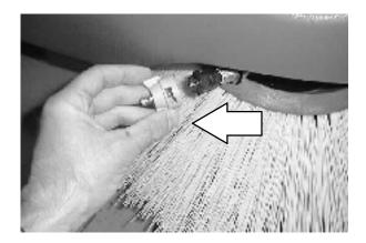
3. Remove the spray nozzle filter screen.
