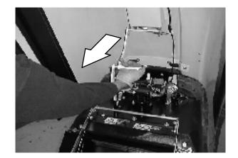
7. Firmly lower the hopper securing bar to lower and release the debris hopper.
