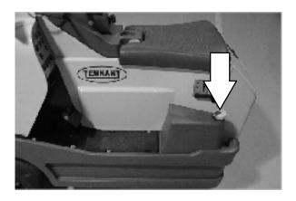
Check the water lines and clamps for damage, tension and wear every 800 hours.
