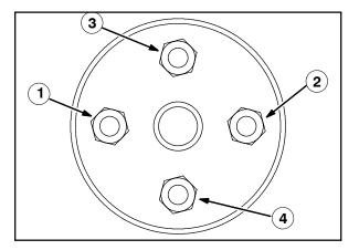
Torque the rear wheel nuts twice to 126–154 Nm (90–110 ft. lbs) after the first 50 hours of operation, and every 800 hours of operation.
