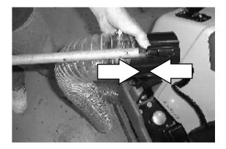
7. Turn the vacuum fan damper handle clockwise to transfer the vacuum power from the main vacuum to the vacuum wand. Turn the handle counterclockwise to transfer vacuum power back to the main vacuum.
