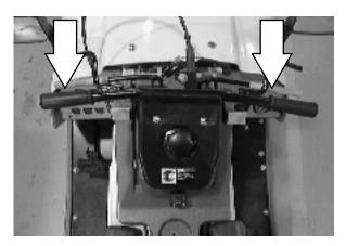
8. Quickly raise the vacuum head control lever when vacuuming large debris, and lower it again.
