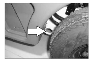
The rear tie-down locations are the bottom lips at each corner of the rear bumper.
