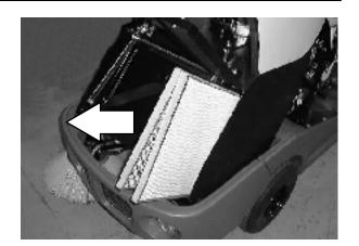
6. Clean the dust filters as required. See the DEBRIS HOPPER section in the MAINTENANCE section of the manual.
