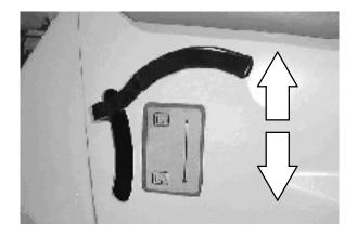
The vacuum head will allow larger debris under the front lip of the vacuum head when it is raised, and will vacuum up the debris when it is lowered.
