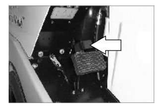
3. Check that the vacuum fan/side brushes switch is in the middle off position.
