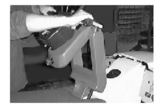
5. Position the steering assembly plate over the rear notched steering plate.
