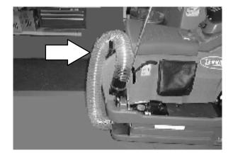
9. Place the vacuum hose and handle back in their storage positions when not using the machine.
