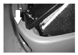
10. Hold up the hopper cover while pushing the prop rod in.
