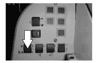
4. Move the throttle lever to the middle engine throttle position.
